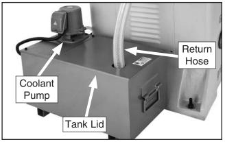
Figure 48. Coolant tank components.
